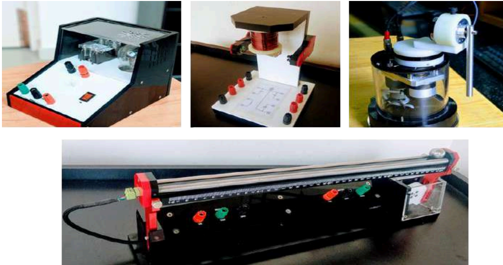
Control Systems Lab, In Clockwise Order from Top: Temperature Control, Magnetic Levitation, Inverted Pendulum and Ball and Beam Balancing
